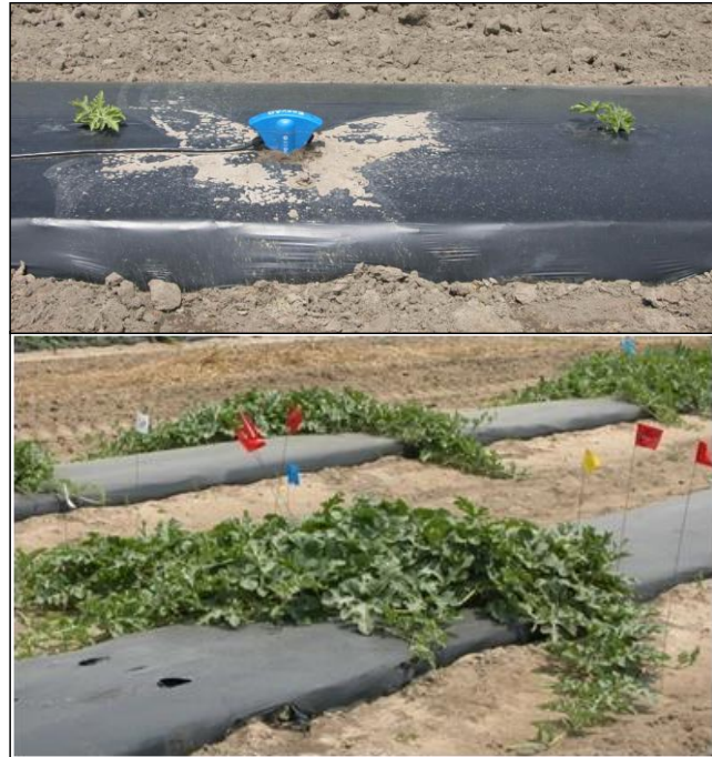
Fig. 1. Capacitance probe located adjacent to the drip line that is below the plastic mulch (top), blooms tagged on 29 May, 2008 (bottom).
